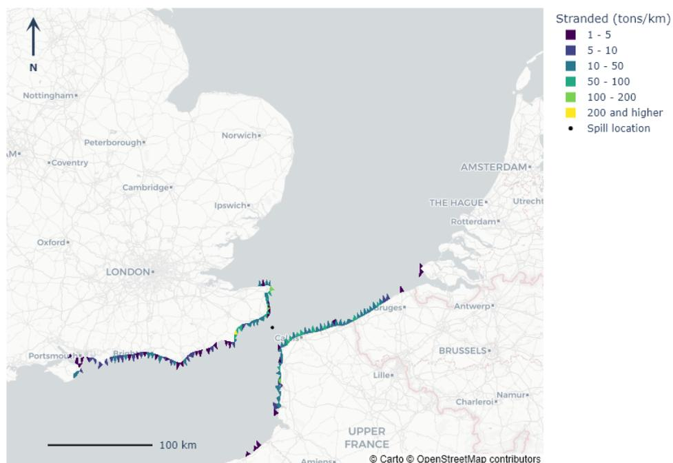
**Figure 4.13** The potential amounts of non-dissolved VLSFO that may possibly be transported to the coast after the assumed spill in the exposure scenario: Collision in the English Channel. The coloured marks indicate the worst-case for each specific point at the coastline, and the indicated amounts of VLSFO stranding on the coast cannot occur in all points.
